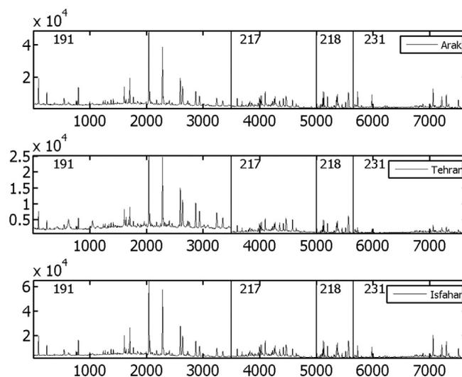
**Fig. 1.** Biomarker fingerprints consisting of combined SICs of terpanes ( $m/z$  191), steranes ( $m/z$  217, 218) and triaromatic steroids ( $m/z$  231) for an untreated soil sample from Arak refinery (upper), Tehran refinery (middle), and Isfahan refinery (lower).
