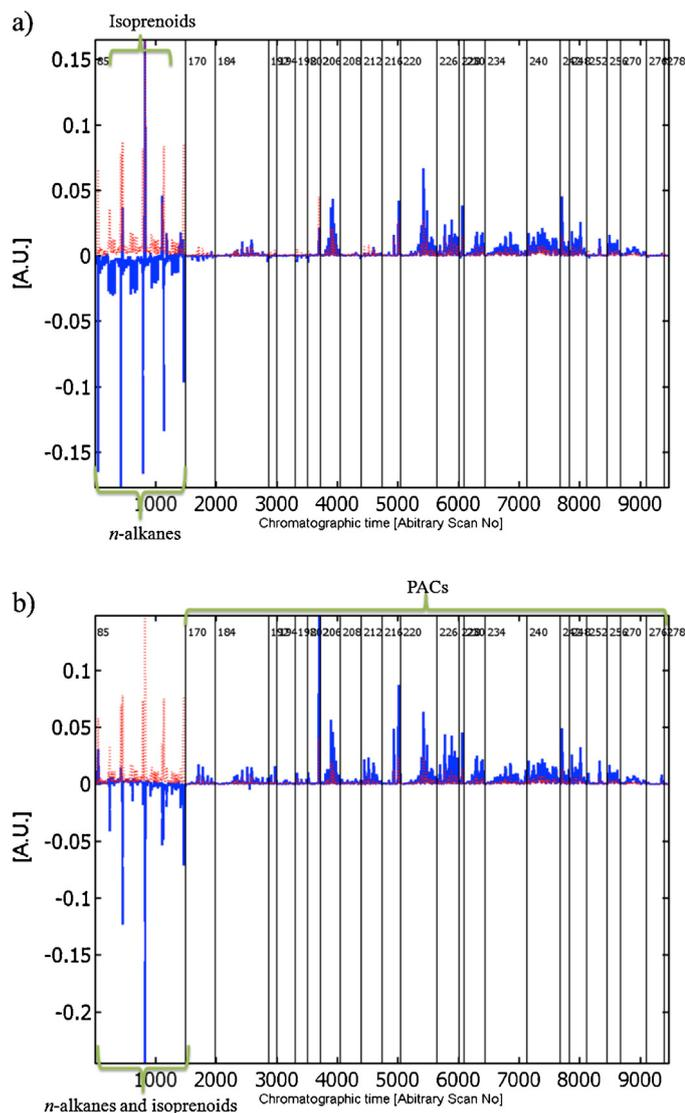
**Fig. 5.** Loading plots: PC1 (a, upper) and PC2 (b, lower) for the PC model of mean-centred data normalization to Euclidean norm after combining SICs (normalization scheme I). The dotted red lines are the mean chromatogram of the entire training set, while the solid blue lines are the loadings. The  $m/z$  groups are specified in loading plot.
